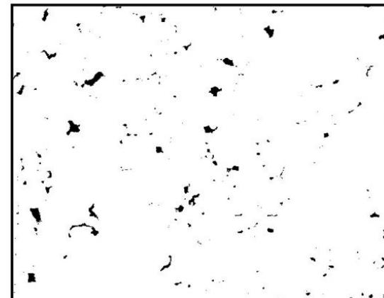
SEM images of a CMX membrane surface before (a) and after (b and c) its operation under overlimiting current during 100 h (b) and 150 h (c).
